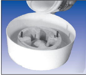
Pouring Replicast Around a Model
