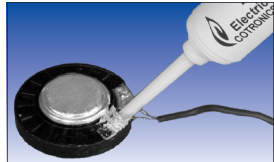
Duralco™ 120 Bonds Leads to an Instrument Assembly
