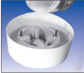
Pouring Replicast Around a Model
