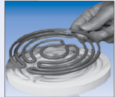
Placing Heater Coils in Insulating Disk
