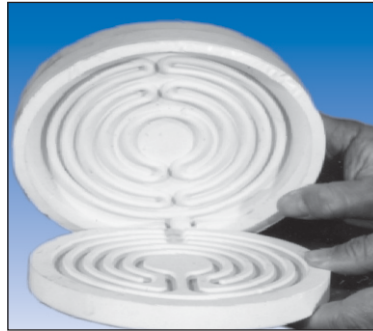
Removing 740 Insulating Plate From Mold
