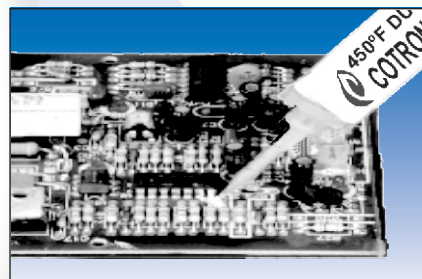
Duralco™ 125 Replaces Soldering on a Circuit Board
